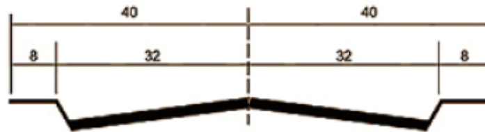
Four-Lane Undivided Roadway 80' R/W Secondary Arterial
